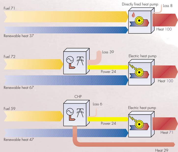
Figure 4: How heat pumps save energy.
