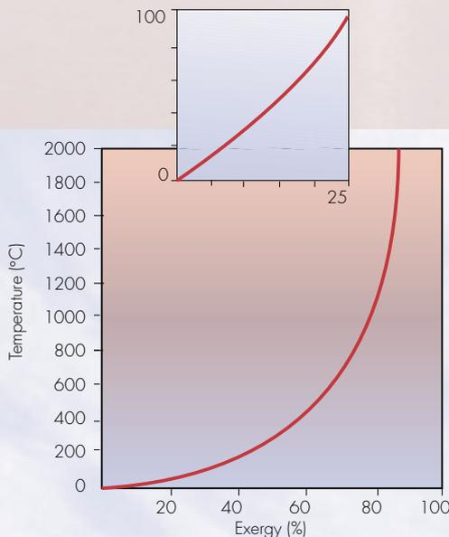
The formula shows that the exergy of heat depends not only on its own temperature, but also on that of the environment – the ambient temperature. Heat can only “do something” when it flows at a temperature above ambient. The kWh released by your house has lost its value completely when it reaches the ambient temperature outside.
